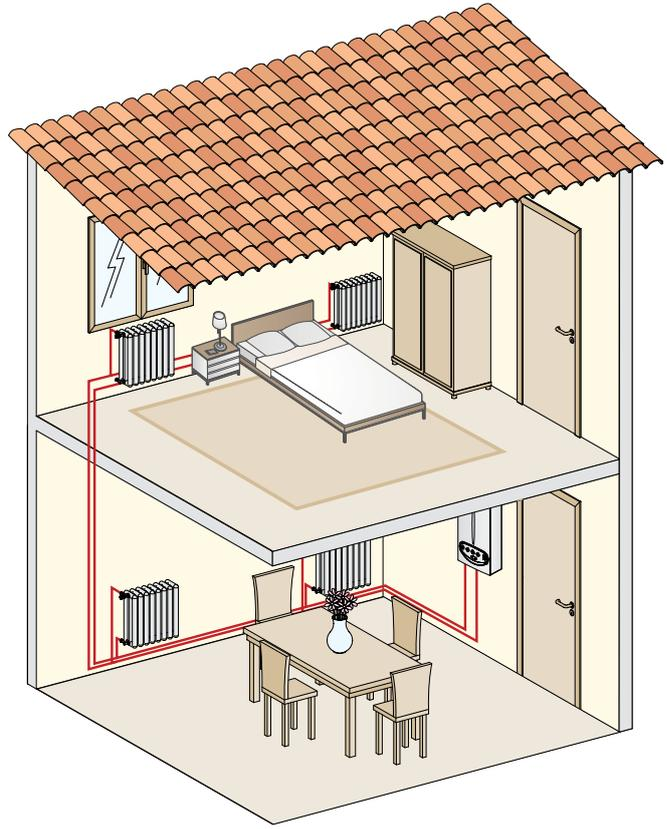
The example above displays a heating only boiler with hydronic radiators to the ground and first floors.
