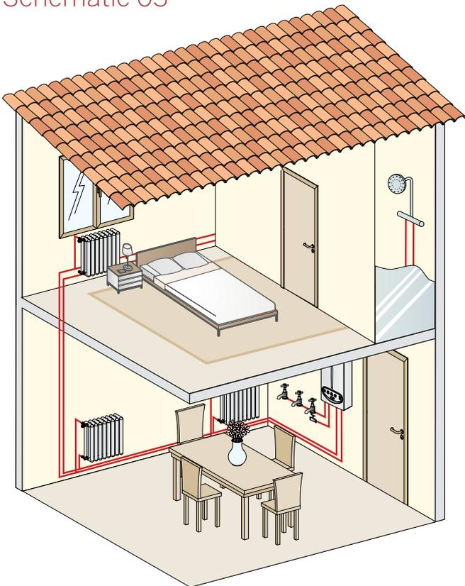
The example above displays a combination boiler providing hydronic heating and an instantaneous domestic hot water solution.
