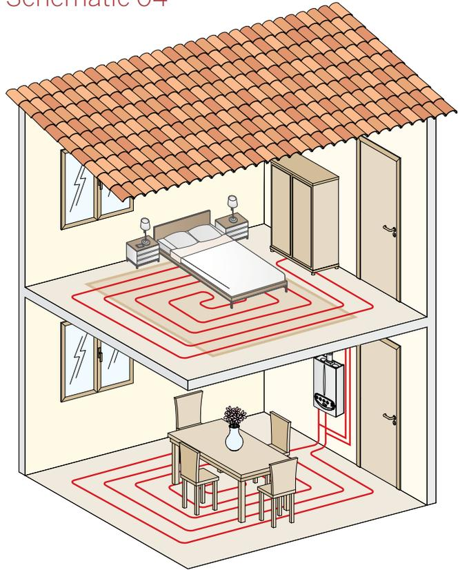
The example above displays a heating only boiler with a hydronic underfloor heating solution to the ground and first floors.
