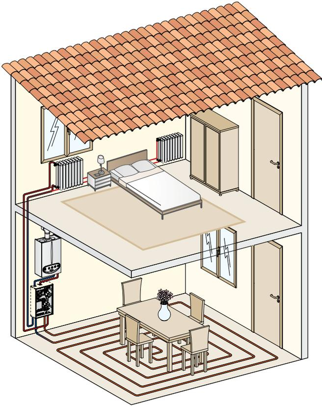
The example above displays a heating only boiler with a multi -zone solution providing underfloor heating to the ground floor and hydronic steel radiators to the first floor.
